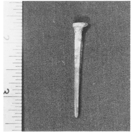
Fig. 2. Early machine-cut clapboard nail from west wall of original Rider-Wood House, Strawberry Banke, New Hampshire, c. 1800-03. Produced by early hand-powered or water-powered machine. Hand-headed. Burrs on opposite-side edges, skewed shank, and rounded end.
