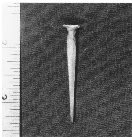
Fig 3. Early machine-cut lath nail from original stairwell of Spencer-Pierce-Little House addition, Newbury, Massachusetts, c. 1800-05. Cut and headed by early two-operation machine. Burrs on opposite-side edges, "neck" under flat, irregular head, rounded end.
