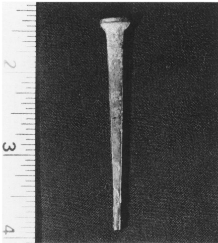
Fig. 7. Nail from original roof sheathing of Custom House, Salem, Massachusetts, 1818. Cut and headed by transitional one-operation machine. Burrs on same-side edges, thick uniform head, bevel under head instead of "neck."
