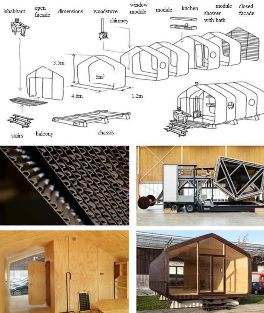
Fig. 7 – Wikkelhouse (package house) made of 24 layers of corrugated cardboard (Photos and information taken from http://www.fictionfactory.nl/en/wikkelhouse/ and http://www.wikkelhouse.com/ accessed on 18.03.2020).
