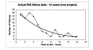
Figure 1 shows a decline in the failure rate from Nis inclusions in 1 major building monitored.
