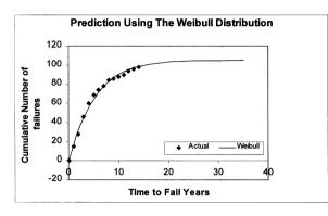
Figure 2. Weibull distribution used to predict future NiS induced failure in tempered glass. It could be predicted that a further 6 to 7 failures could occur over the next 25 years.
