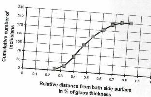
NiS can only cause breakage when situated in the tensile zone of the glass. In the compressive zone, the stress initiated by NiS is (over)-compensated. Between the two extremes exists a transition zone where NiS stones are partly unable to break the glass.
