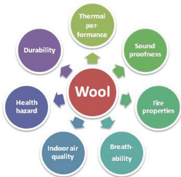
Fig. 1. Key properties of wool as insulation material.
