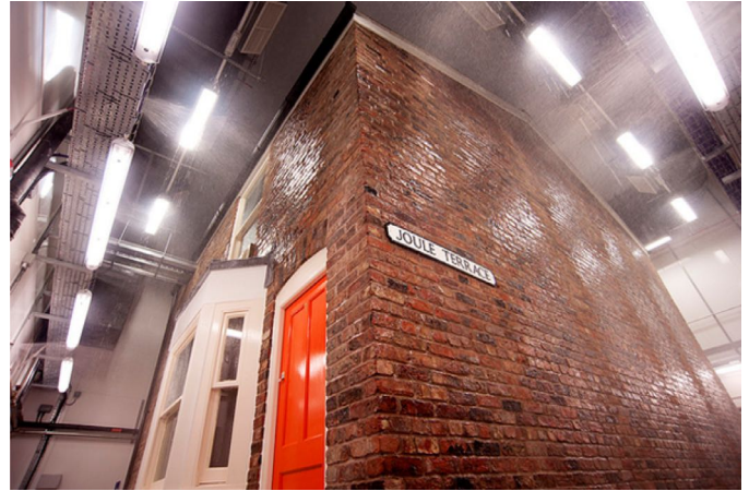
Fig. 2. Energy House of the University of Salford. It is a full size typical Victorian House build inside a climate chamber.
