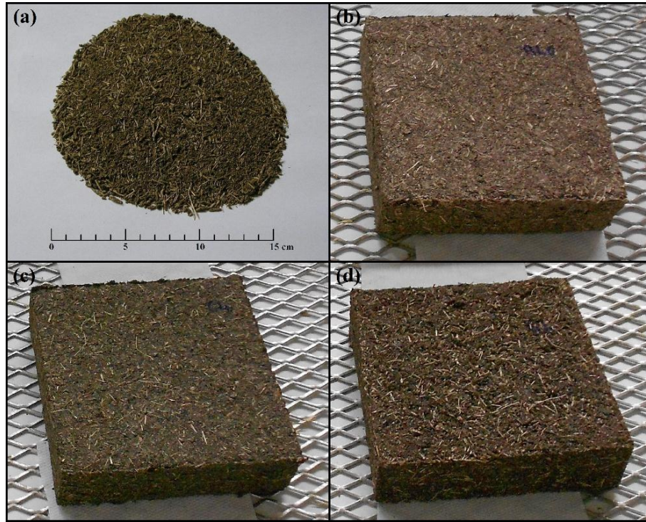
Figure 2. Photographs of the cake (a) and of the three fiberboards with 25% binder content (b, board S4; c, board C4; d, board G4).
