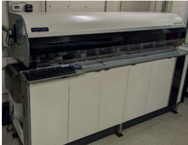
Figure 7.17. Autoline Supplied by Lorentzen & Wettre Products (now ABB).
