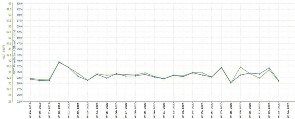
Figure 7.20. Trend between RCT tested in lab vs RCT predicted
