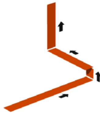
Laying direction of the joint insulation tape around the window sill and to the window.
