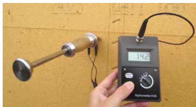
Board moisture content \leq 19,5\% with a setting for spruce/pine.
