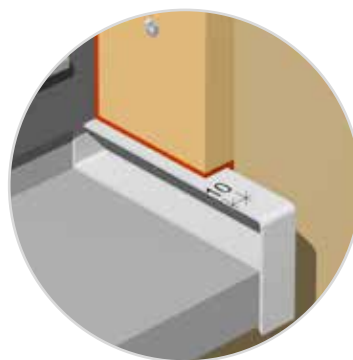
Offset of approx. 10 mm for render applications.
