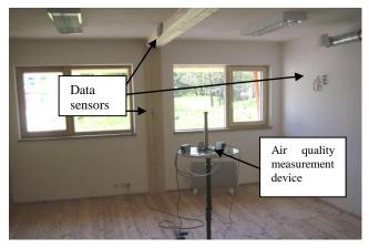
Figure 2: Realized wooden building module inside of the framing and clay module during air quality measurements
