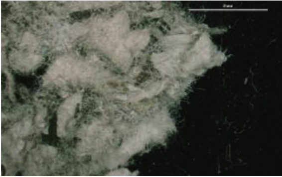
Fig. 2. Microscopic scan of cellulose fibres, 10X magnification.
