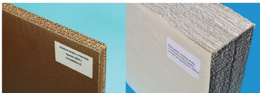
Fig. 2: Thermal insulation boards based on an old corrugated carton.
