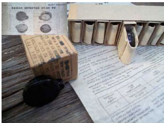
FIG. 30.2 A set of ten original DT-60 dosimeters packaged with instructions and specifications. The box is dated 1951, and the dosimeters were manufactured by the Polaroid Corporation. They are sold as ‘a Cold-War beauty’, which ‘shows you just how fried you are after a radiation exposure’ (source: Omaha’s Surplus 2016)
