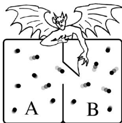
FIG. 20.4 'Boxed-up Ghosts'. Maxwell illustrated with a demon how the second law of thermodynamics could be violated. The demon was the gatekeeper.
