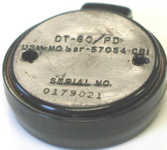
FIG. 30.1 The photograph shows an open glass DT-60 personnel dosimeter used in the 1950s and 1960s. It was placed in a circular plastic container that opened only with a special tool to protect sensitive radiation data (source: ORAU, Health Physics Historical Instrumentation Museum Collection)
