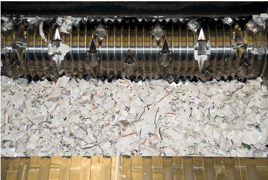
FIG. 22.4 The paper shredder's metal 'teeth', spinning shaft, and paper fragments produced. Friesens Corporation, Altona, Manitoba, Canada, 2011 (photo by Rosemarie and Pat Keough; reprinted with permission from Rosemarie and Pat Keough)
