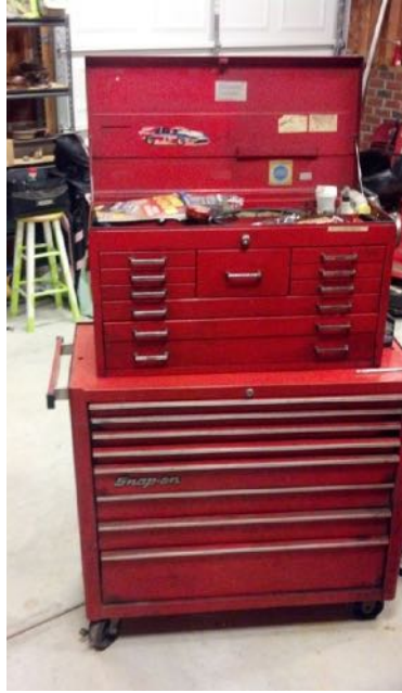
FIG. 35.1 This example of a tool chest, often referred to as a Highboy Tool Chest, is of a type commonly found in professional and amateur garages and workspaces. This particular eighteen-drawer steel chest was constructed in the 1990s by Snap-On and was in use until 2015. The chest consists of two pieces, with the lower portion resting on casters for mobility. While the chest has been retired, remnants of the previous owner's personal items can be seen in the top of the chest (photo by Don Duprez)
