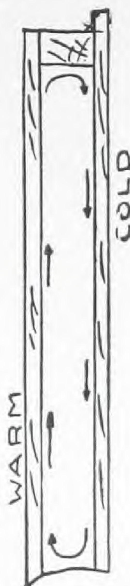
Drawing showing heat conduction by air currents in built-up air spaces.
