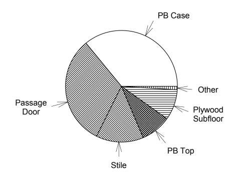
Fig. 1 Fractional contributions of indoor sources to whole-house formaldehyde emission rates
