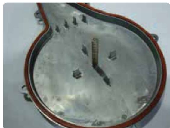
Figure 136 Heat exchanger cover plate removed
