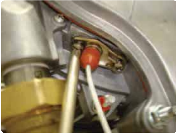
Figure 133 Removal of Ignition electrode
