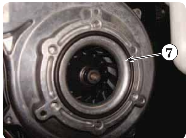
Figure 16 Insure "O" ring is in place.
