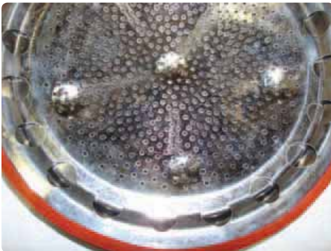
Figure 138 Inspecting interior and cleaning the burner
