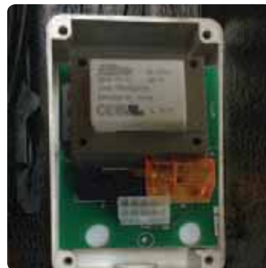
Figure 61 Thermostat-Relay box terminals Combi and Central Heating boilers
