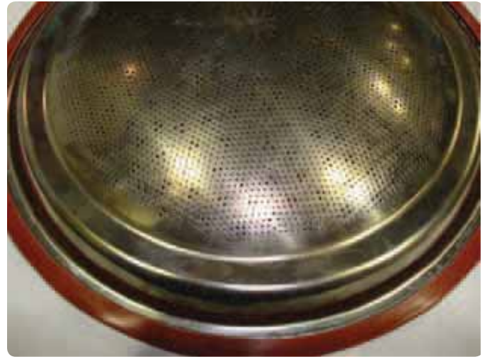
Figure 139 Inspecting exterior and cleaning the burner
