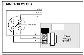
ALTERNATE WIRING: If you choose to wire the feeder to a separate power source from the burner circuit, do not install jumper between 2 and 3. Connect a wire from the "Feed" terminal on the water feeder to terminal 4 on the low water cut-off. Connect a wire from terminal H on the water feeder to the hot side of the power source. Connect a second wire from terminal H to terminal 3 on the cut-off. Connect a wire from terminal N to the common side of the power source.
