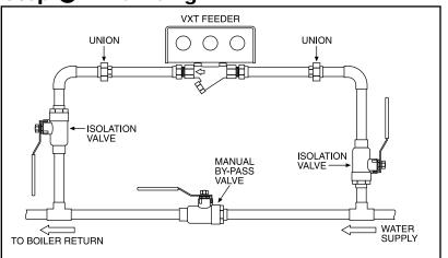
Feeder must be installed with a manual by-pass. Use isolation valves and unions to allow easy removal for service or replacement. *Note:* Arrow on VXT valve indicates direction of water flow.
