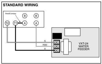
**ALTERNATE WIRING:** If you choose to wire the feeder to a separate power source from the burner circuit, do not install jumper between T1 and A. Connect a wire from the "Feed" terminal on the water feeder to terminal A on the low water cut-off. Connect a wire from terminal H on the water feeder to the hot side of the power source. Connect a second wire from terminal H to the other terminal A on the cut-off. Connect a wire from terminal N to the common side of the power source.
