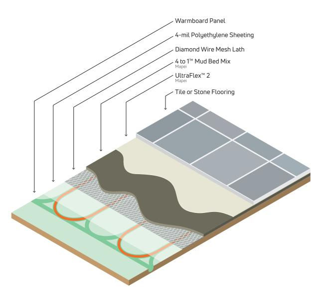
Surface temperatures of the finish flooring should not exceed 85°F.
