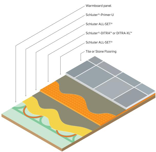
For stone applications over DITRA, structural joist (TJI) **MUST** be on 16" centers.
