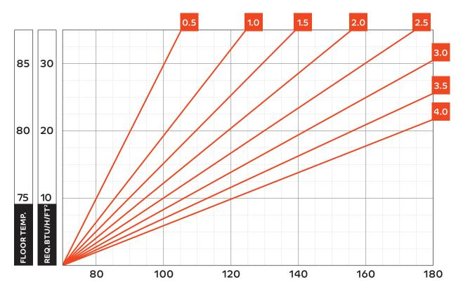
Average of Supply/Return Water Temperature at Manifold for Good Dynamic Performance
