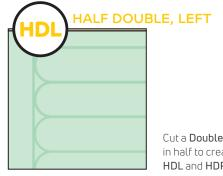
Cut a Double Panel in half to create the HDL and HDR panels.
