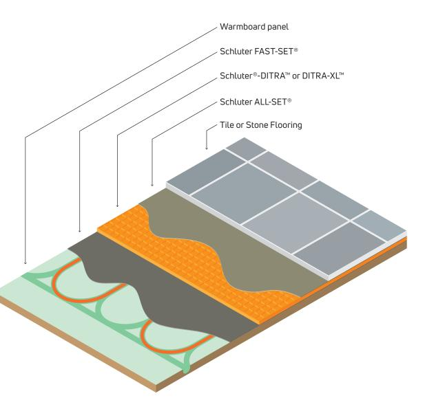
For stone applications over DITRA, structural joist (TJI) **MUST** be on 16" centers.
