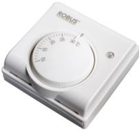
Individual room thermostats in your house measure the temperature of the air in the room, if it is cold it will tell the central heating to turn on, when it gets too warm it tells the central heating to turn off. Room thermostats need a free flow of air to sense the temperature, so they must not be blocked by curtains or furniture, or put near heat sources.
