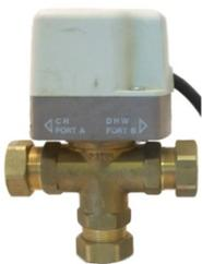
This component is responsible for choosing where the water from the boiler goes. The valves have a motor attached to the top so they are able to control the flow of heating water to either the central heating or hot water system. They come in two main types, 2 port or 3 port valves.
