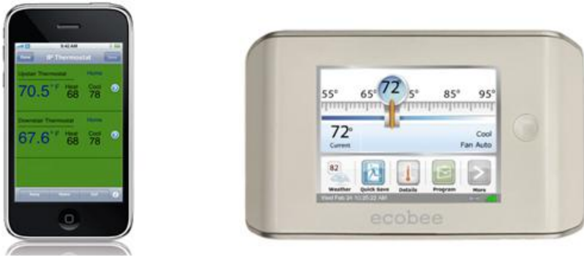
Figure 3: From left: iPhone app for thermostat control, and an Ecobee Internet thermostat (Source: http://www.smarthome.com/iphone_thermostat_control.html , http://www.ecobee.com/product/smart-overview/ )
