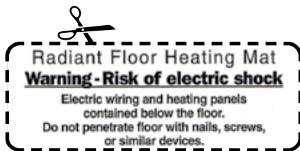
This electric radiant heating warning label must be cut out and taped near or on the face of the control.
