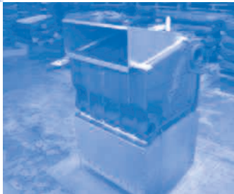
Cast iron section assembly with flue collector/draft hood installation
