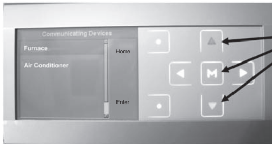
FIGURE 74 NAVIGATE TO FURNACE AND SELECT.
