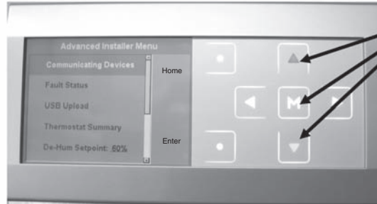
FIGURE 73 NAVIGATING TO COMMUNICATING DEVICES AND SELECT.
