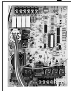
INTEGRATED FURNACE CONTROL
