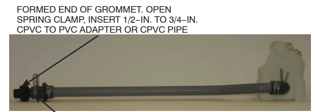
FRONT VIEW LEFT SIDE DRAIN PIPE ORIENTATION FOR CONDENSATE DISCHARGE NOTE: Remove Inducer Housing for easier access, if desired.
