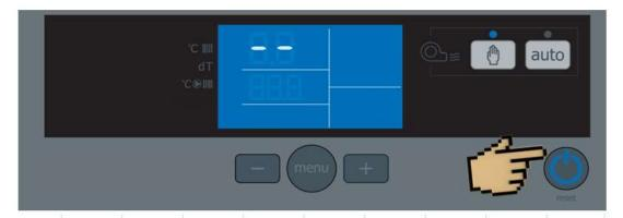
When the control panel is switched ON, fan will not operate, but all safety functions are active. You
