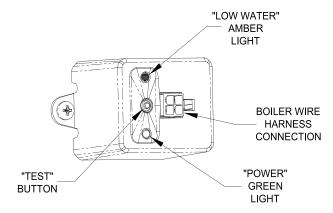
Figure 10.1: IDL 1200 Low Water Cut-Off
