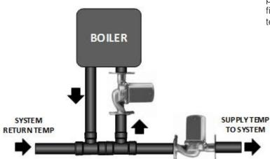
This is an improvement over simple by-pass piping to reduce condensation. Again this is a fixed system. It can not adapt to variations in temperature and flow.
