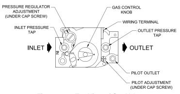
Figure 10.2: Top View of Gas Valve
