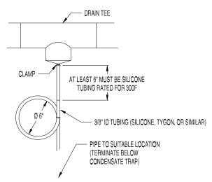
Figure 6.12: Condensate Trap/Drain Detail
