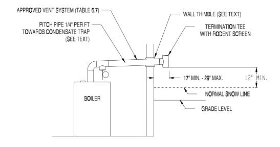
Figure 6.2: Horizontal Direct Exhaust Vent System (Vent Options 1, 2)
