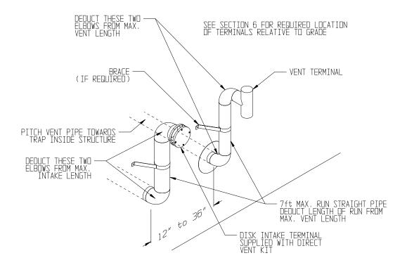
**Figure A.5: Horizontal Terminal Offsets**
