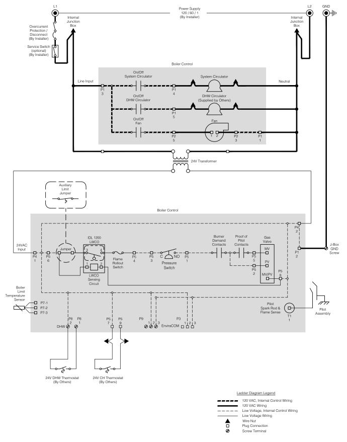
Figure 9.4: Wiring Ladder Diagram
