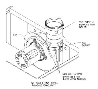
Figure 6.10: Installation of Vent Adapter
