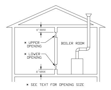
Figure 5.1: Indoor Combustion Air Method
