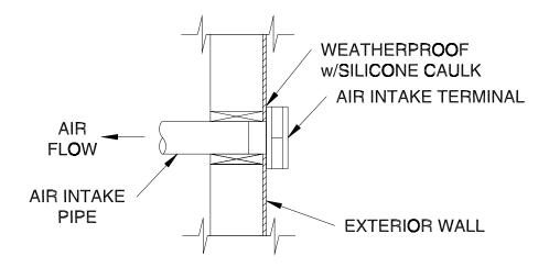
Figure A.3: Horizontal Installation of Air Intake Terminal
