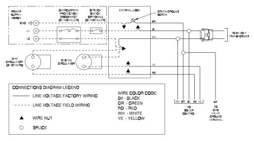
Figure 9.1: Line Voltage Connections
