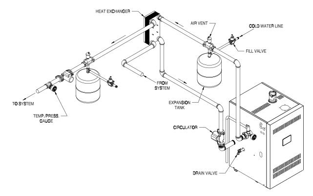
Figure 7.4: Isolation Of Boiler From System With A Heat Exchanger
