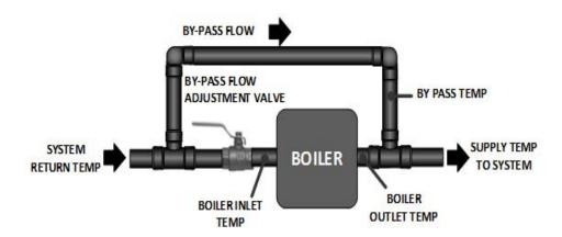
Regardless of by-pass flow, boiler will have inlet temperatures that are same as system return temperature. When boiler inlet temperatures fall below 120°F, boiler will condense. As by-pass flow is increased less water flows through boiler, which increases boiler temperature rise. This will help reduce propensity for condensation but will not stop it.
