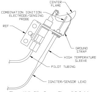
Figure 10.7: Pilot Burner Flame (LP Only)
