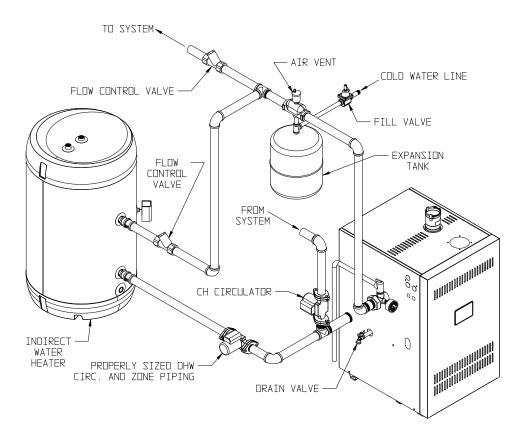
Figure 7.3: Indirect Water Heater Boiler Side Piping
