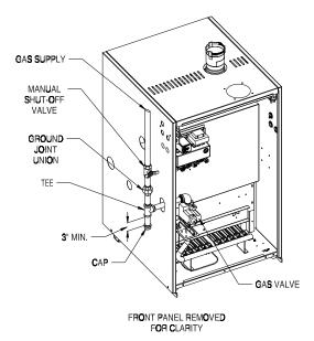
Figure 8.1: Gas Connection To Boiler
