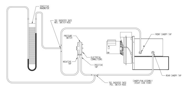
Figure 12.3b: Measuring Pressure Across Pressure Switch
