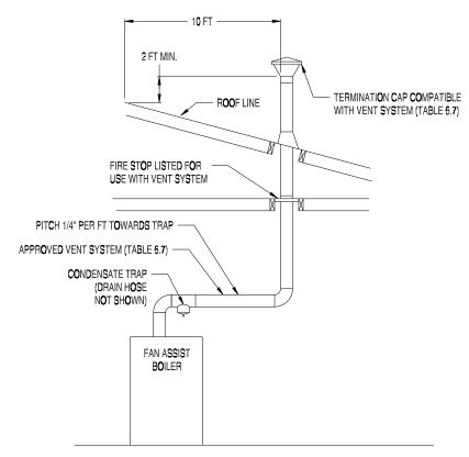
Figure 6.6: Vertical Direct Exhaust System (Vent Options 3, 4)
