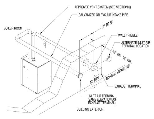
Figure A.4: Horizontal Direct Venting (Vent Options 5-7)
