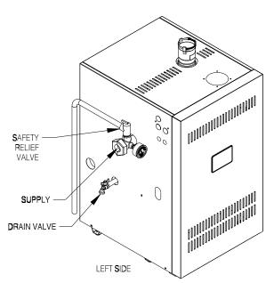
Figure 7.1: Standard Safety Relief Valve Position
