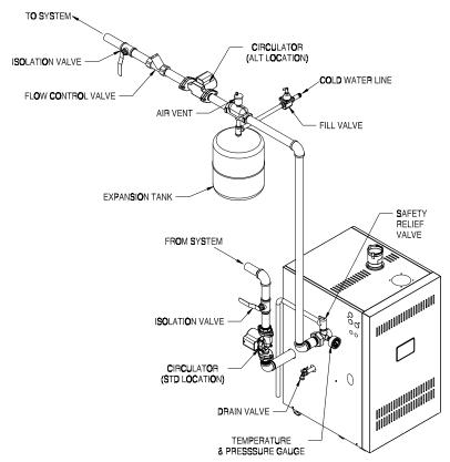
Figure 7.2: Standard Boiler Piping
