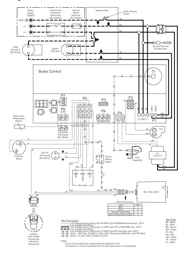
Figure 9.3: Wiring Connections Diagram
