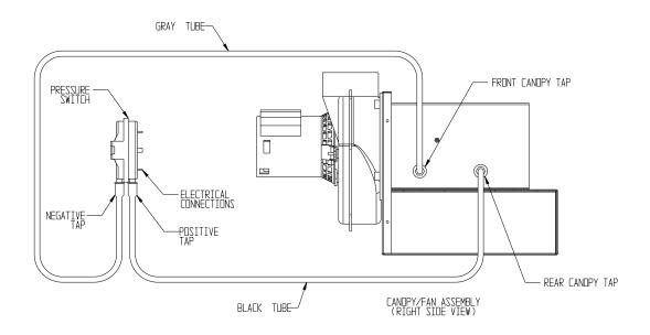
Figure 12.3a: Pressure Switch Connections
