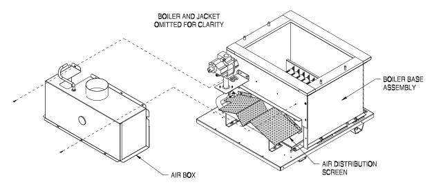
Figure 12.1: Direct Vent Air Box Removal
