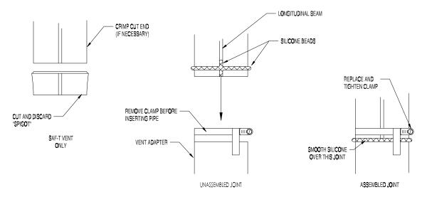
Figure 6.11: Connection of First Vent Pipe to Boiler Vent Adapter
