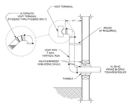
Figure 6.5: Optional Terminal Offset for Horizontal Vent Systems
