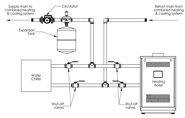
Figure A-1: Isolated Boiler from Refrigeration System
