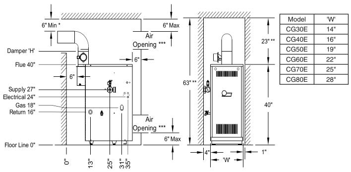
Figure 1-3: Minimum Closet Clearances
