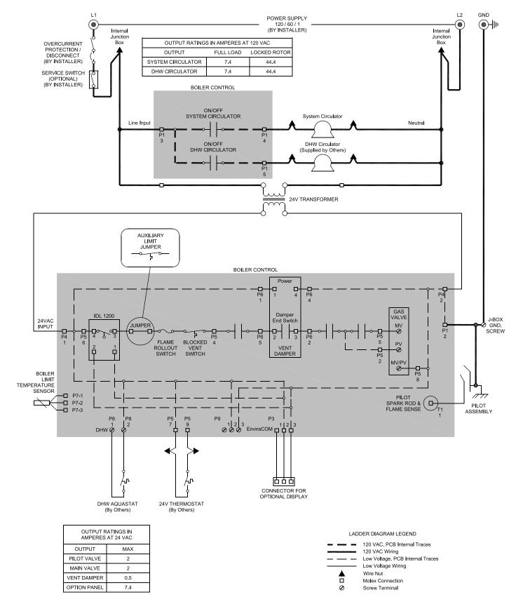
Figure 8-2: Schematic Ladder Diagram
