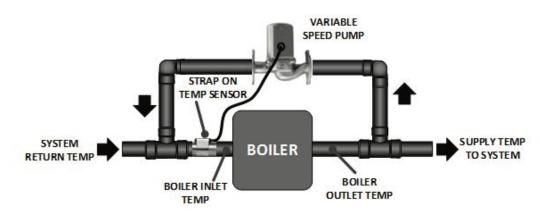
A strap on temperature sensor measures boiler inlet temperatures. This temperature signal is sent to a variable speed pump that will ensure boiler inlet temperatures are always greater than the factory by-pass kit set point of 120°F.
