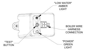
Figure 9-1: IDL 1200 Low Water Cut-Off
