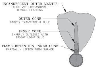
Figure 9-6: Main Burner Flame
