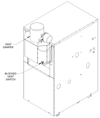
Figure 5-1: Vent Damper Installation
