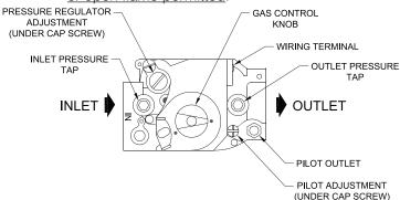
Figure 9-3: Top View of Gas Valves
