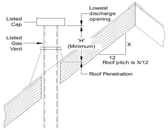
Figure 5-3: Termination Location for Gas Vent
