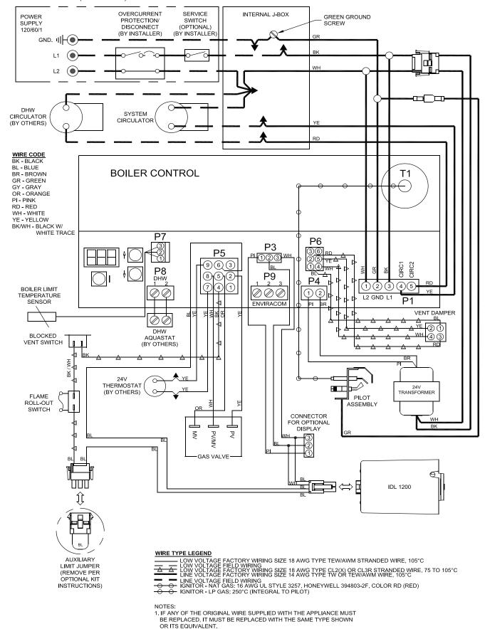
Figure 8-1: Wiring Connection Diagram
