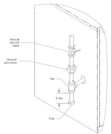
Figure 7-2: Pilot and Gas Piping
