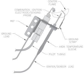
Figure 9-5: Pilot Burner Flame (LP Only)
