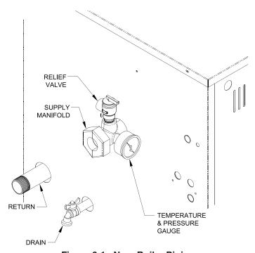
Figure 6-1: Near Boiler Piping
