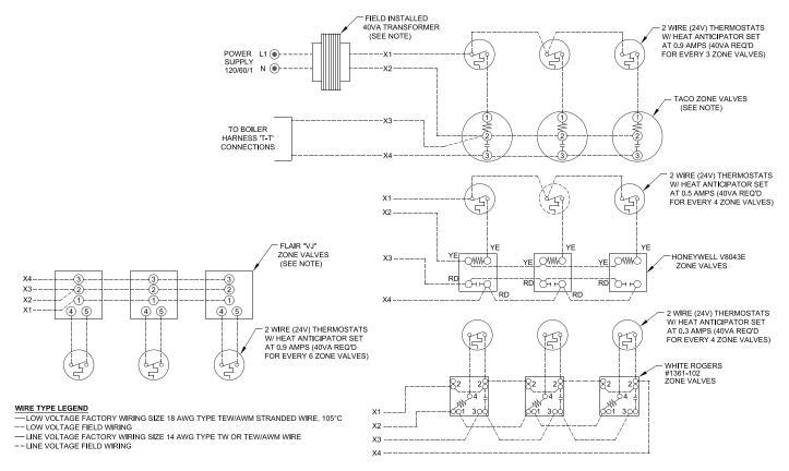
Figure 8-3: Wiring Schematic, Zone Valves
