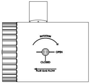
Figure 5-2: Vent Damper Position Indicator
