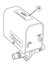
2. Uni-Match water feeders are shipped from the factory equipped for a 2 gpm feed rate. A separate kit with instruction sheet and field installable orifices for 1 gpm and 4 gpm feed rates is included. If the alternate feed rates are required, refer to the instruction sheet provided with the kit for orifice replacement.
