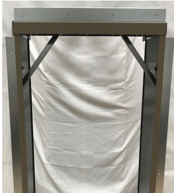
Figure 11 - Wall sleeve installed from outside angle 3
