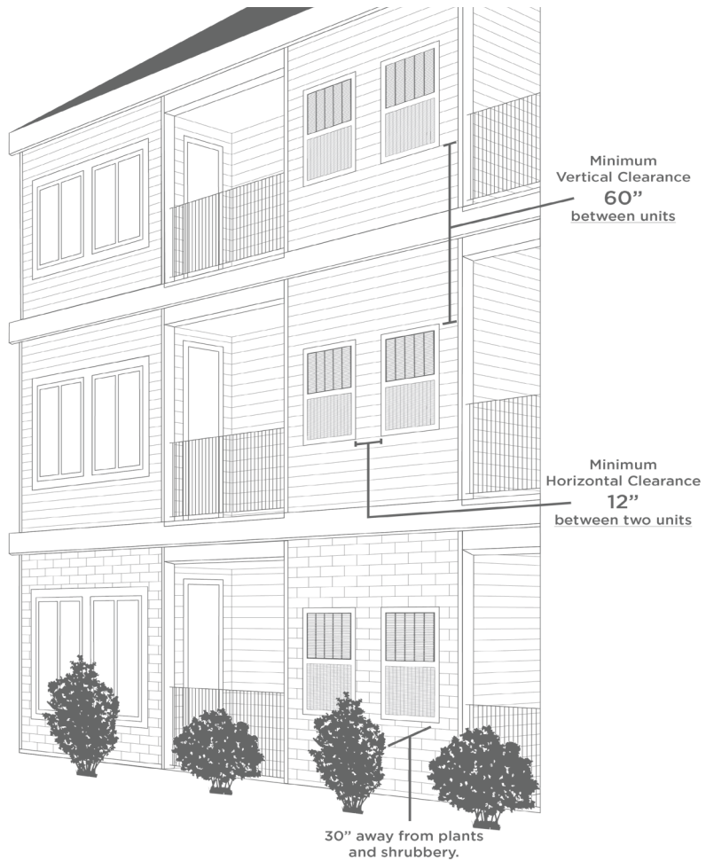
Fig 4: Building Clearance Needed
