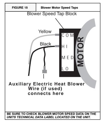
**NOTE:** On Heat Pumps Electric heater blower wire must be attached to the same speed tap required for cooling/heat pump operation. **See FIG-URE 11 notes.** The **yellow** lead **MUST** always be connected to the speed tap block at the common quick connect terminal. The terminal is identified as **COM**.
