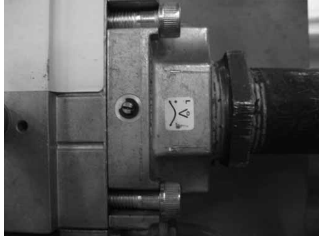
KN-30 High Fire CO 2 Adjustment Screw - Clockwise = Decrease Counterclockwise = Increase
