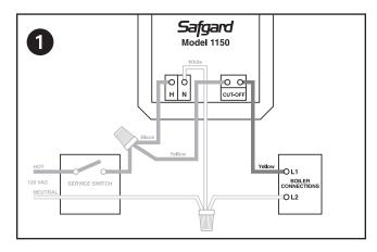
**Step 3** Connect the second yellow wire (CUT-OFF) from the Safgard 1150 to the (L1) boiler connection.
