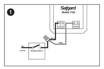
**Step** ① Connect the black wire (H) and one of the yellow wires (CUT-OFF) from the Safgard 1150 to the hot 120 VAC lead coming from the service switch.
