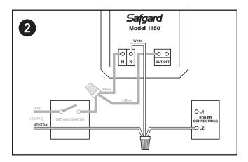
**Step 2** Connect the white wire **(N)** from the Safgard 1150 to the neutral 120 VAC lead and to the **(L2)** boiler connection.
