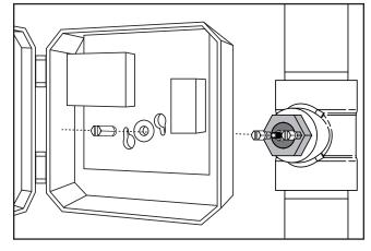
Mount the control box on the probe by aligning the keyhole slots with the two extended nuts. Replace the center extended nut. Secure the control box by tightening all three extended nuts.
