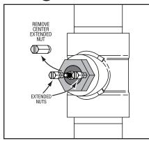
Remove center extended nut. Apply pipe sealing compound to probe threads and install in boiler or tee. Tighten so that the two smaller extended nuts are horizontally aligned.
