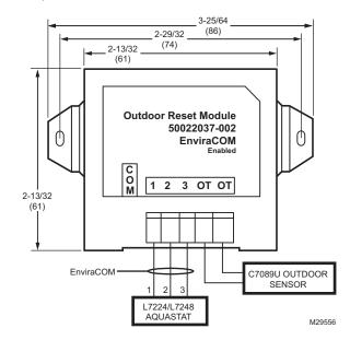
Fig. 1. 50022037-002 Outdoor Reset Module wiring diagram.
