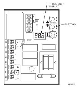
Fig. 2. Location of L7224/L7248 3-digit display and buttons.
