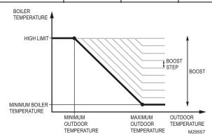
Fig. 3. Outdoor temperature setback curve with boost.
