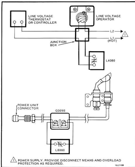
Fig. 4—Typical wiring hookup for line voltage system.
