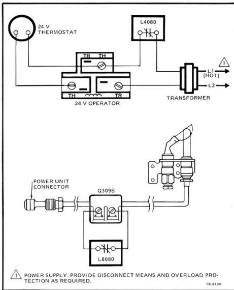
Fig. 3—Typical wiring hookup for 24 V systems.
