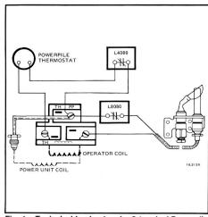
Fig. 1— Typical wiring hookup for 3-terminal Powerpile control systems.
