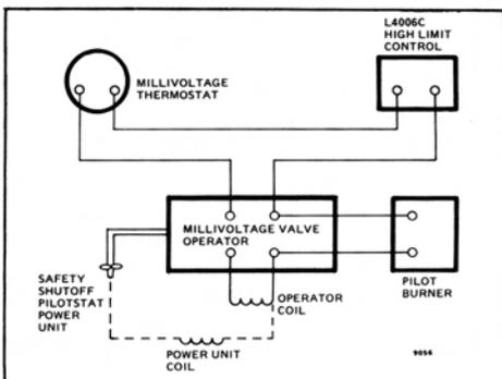
Fig. 8—Typical Powerpile system wiring diagram, using L4006C.
