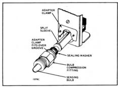
Fig. 3— Direct immersion model with bulb compression fitting partially removed.
