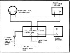
Fig. 8— Typical Powerpile system wiring diagram, using
