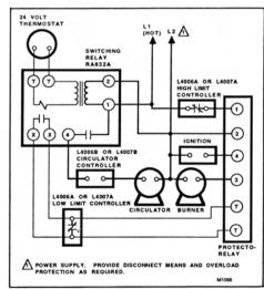
Fig. 5— Hookup for oil-fired, summer-winter hydronic system with domestic hot water using L4006A or B, L4007A or B. This is typical where control for domestic hot water is added, or where each Aquastat controller is mounted in a separate location.
