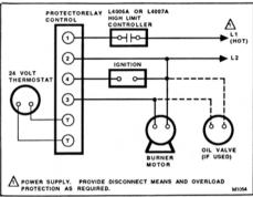
Fig. 4—Typical hookup for oil-fired gravity system, using L4006A or L4007A.
