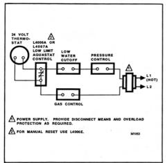
Fig. 6—Typical hookup for gas-fired system with domestic hot water, using L4006A,E or L4007A.
