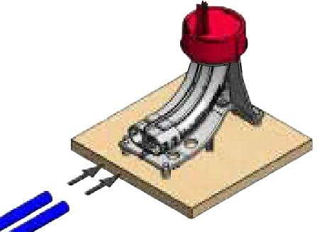
**INSERT 1/2" PEX TUBES THROUGH 703 BODY.** (FIG. 3A) Note: For 8" slab height PEX tubing should extend 8-5/8" beyond corrugated sleeving, prior to PEX insertion into bracket.
