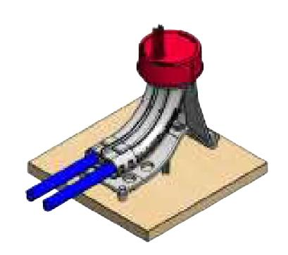
PUSH TUBES THROUGH UNTIL IT HITS BOTTOM SIDE OF CAP. (FIG. 3B)
