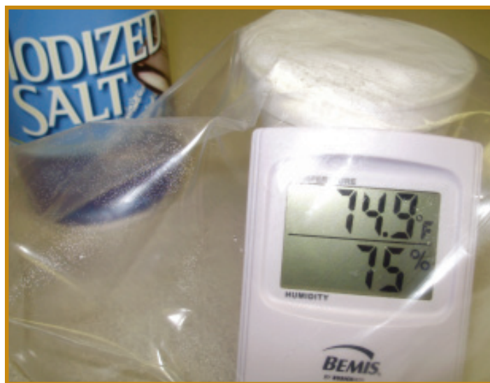
Figure 3. Salt solution calibration test, 75 percent humidity. (Photo by Carl Pedersen)
