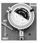
The light portion of the clock face represents the morning and afternoon (6 a.m. to 6 p.m.). The dark portion represents the evening and night (6 p.m. to 6 a.m.). The arrow located directly beneath the time dial face that is marked "TIME" must always point to the correct time of day. To adjust dial for correct time of day turn dial in clockwise direction **only** (as indicated by arrows on dial), never turn counter
