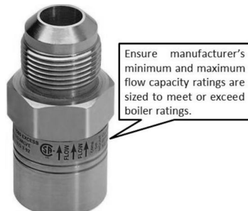
Figure 48 - Excess Flow Valve (EFV)
