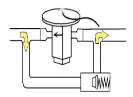
Most expansion valves used in current Goodman/Amana® Brand Heat Pump products use an internally checked expansion valve.
