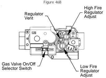
Honeywell Model VR9205 (Two-Stage) Figure 47A
