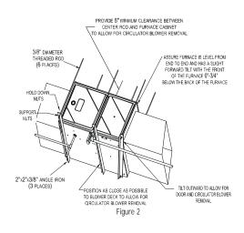
When installing a furnace horizontally, additional consideration must be given to the following:
