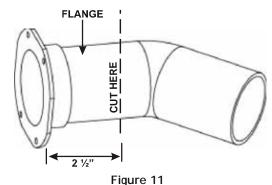
Vent/Flue Pipe Cuts
