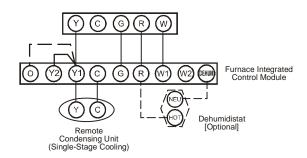
NOTE: To apply a single stage Heating Thermostat, the thermostat selector sqitch on the Integrated Control Module must be set on sinle-Stage.
