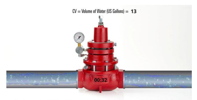
The volume of water at 60°F that will flow through a valve, per minute, with a pressure drop of 1 psi across the valve.
