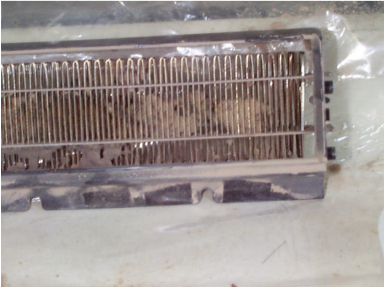
Figure 4: Heater A Heating Element
