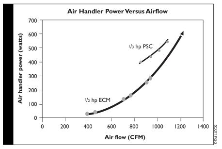
**Figure 1.** The air flow range of the furnace with the ECM extends beyond that shown in the figure, but the furnace powered by the PSC motor is limited to the four speeds shown. The two 60,000 Btu/hr furnaces operated in similar static pressure environments.
