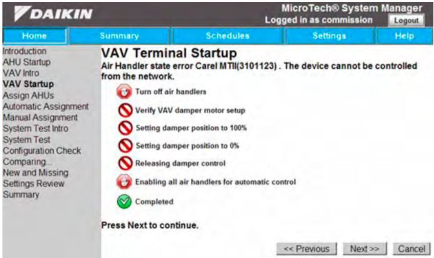
Figure 19: VAV Terminal Startup
