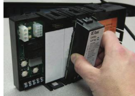
Insert OCP LWCO Card into selected slot
