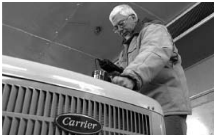
Carrier units are sound tested in accordance with ARI Standard 270.
